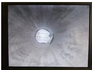
LED illumination inside a Stainless steel p Pipe Inner Diameter: 33mm Length 20cm
