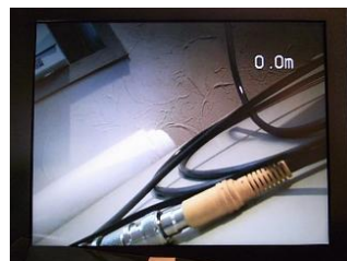
Bright Room (LED OFF) 12cm to the connector 40cm to the back wall
