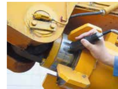
Diagnosing wear and tear using hardness measurements
